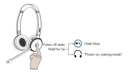
2. Connect the WDD60 to a PC or desk phone and put the WDD60 into pairing mode.
