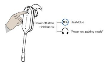
2. Connect the WDD60 to a PC or desk phone and put the WDD60 into pairing mode.
